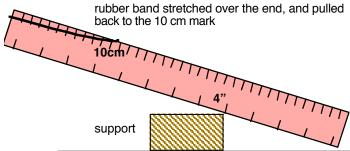
Another variable that will affect your launch range is how far back the rubber band is stretched. For each rubber band launch, you will need to record **stretch distance**, which is just the distance that the rubber band was stretched back (10 cm in the diagram here).
